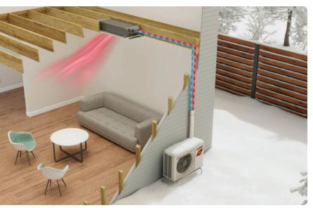
In cooling mode, a heat pump works by moving heat from inside the home to the outside. The indoor unit absorbs and sends the room's heat to the outdoor unit, where it is cooled and returned to the room to provide you with cold air.
